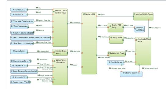
With the context understood, the functional design process produces a functional architecture that develops the product logic that will eventually drive the downstream logical design, providing traceable functional scenarios for product architecture optimization.
