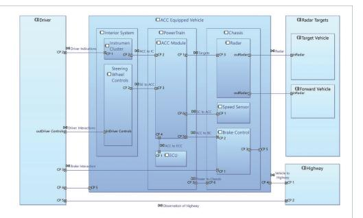
Functional allocation decisions about how/where the functions are accomplished create a logical architecture that drives physical architecture decisions, all of which culminates in a physical system architecture that documents/understands allocation decisions and system interfaces/exchanges in context of the operating environment that is able to drive the downstream development environments to an integrated solution.
